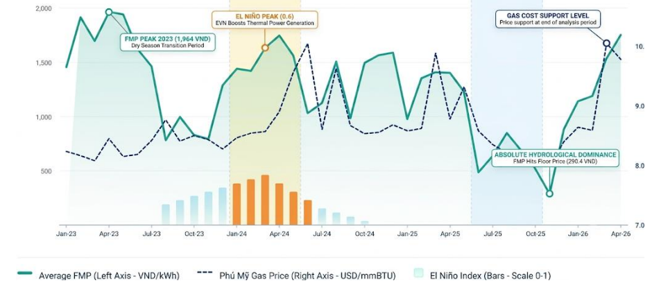
Figure: FMP correlation – hydrology vs. gas prices FMP is driven by fuel costs and hydrological conditions
